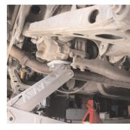
When jacking up the rear of the car, put the jack under the differential. All but the earliest cars (such as this one) have a flat section there that is nice and stable.
