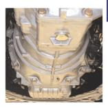
This is the transmission viewed from underneath, looking at the bellhousing bolts. Five are visible in this photo. The clutch slave is on the right side of the bellhousing, pressing on the clutch release fork that is surrounded by the rubber boot.
